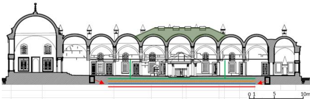
Figure 3.305. Reuse interventions applied on A-A Section of restoration Project made in 2011 (restoration Project from archive of Anfora Architecture)
